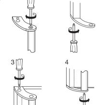
2. Fit the top handle bracket on the top left-hand side of the door (3) and screw the handle rod to the bottom handle bracket (4).
